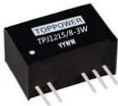
**DESCRIPTION:****5.2KVDC Isolated DC/DC Converters for IGBT drivers**
